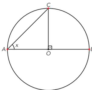
$$x = \text{med}(\widehat{BAC}) = \frac{\text{med}(\widehat{BOC})}{2} = \frac{90^\circ}{2} = 45^\circ$$
